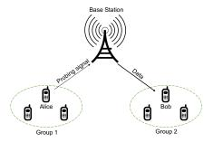
Figure 2: A downlink system with 2 user groups, the BS receives probing signal from Alice and transmits data packets to Bob (channel is already known) simultaneously.
