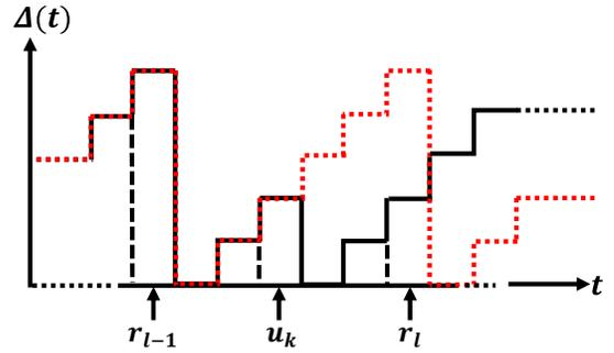
Fig. 10: An illustration of the advantage of a constructed reactive policy  $\pi' \in \Pi^R$  over an arbitrary given non-reactive policy  $\pi \in \Pi \setminus \Pi^R$ , where the solid black curve and the dashed red curve denote the AoI trajectories under policies  $\pi$  and  $\pi'$ , respectively.
