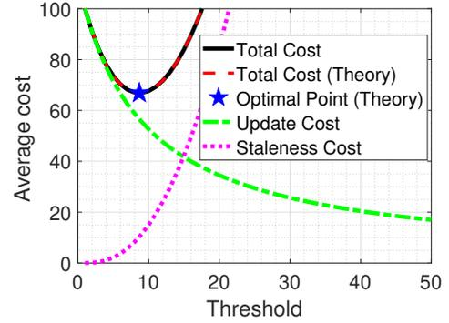
Fig. 5: Average cost under threshold-based policies with different thresholds when  $f(\Delta) = \Delta^2$ , where  $\lambda = 0.1$  and  $p = 100$ .
