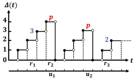
Fig. 2: An illustration of the AoI evolution at the server. There are two updates (in time-slots  $u_1$  and  $u_2$ ) during the process of serving three requests (in time-slots  $r_1$ ,  $r_2$ , and  $r_3$ ).
