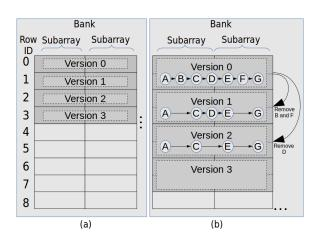
Figure 3: Versions and rows in a subarray of a bank of DRAM. A version may span (a) multiple subarrays and (b) multiple rows. Versions track the evolution of data structures (shown in (b)).
