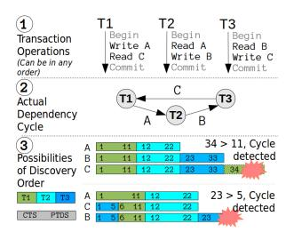
Figure 8: Detecting dependency loops using post-dated *logical* timestamps and an increment of 10. Note that discovery starting from B and C can be made equivalent to the illustrated example through rotating the edge numbers.
