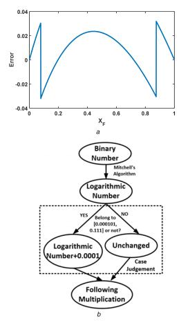
**Fig. 2** *Proposed calibration with case judgement* (a) Error curve, (b) Calibration flow
