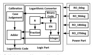
$\textbf{Fig. 3} \ \textit{Block diagram of the proposed logarithmic converter}$
