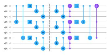
Fig. 3. Encoding and Decoding Circuit of the Shor Code
