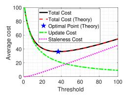
Fig. 4: Average cost under threshold-based policies with different thresholds when  $f(\Delta) = \Delta$ , where  $\lambda = 0.1$  and p = 100.
