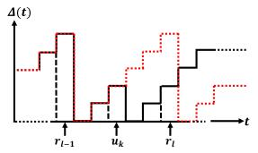
Fig. 10: An illustration of the advantage of a constructed reactive policy  $\pi' \in \Pi^R$  over an arbitrary given non-reactive policy  $\pi \in \Pi \backslash \Pi^R$ , where the solid black curve and the dashed red curve denote the AoI trajectories under policies  $\pi$  and  $\pi'$ , respectively.
